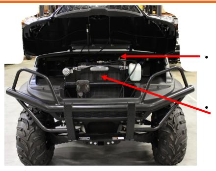
Fresh / clean air is taken in under the dash and passed through the ROPS to provide dust-free air to the CVT Plus transmission Front-mounted radiator provides convenient location and reduced risk of overheating caused by sand and/or mud clogging
