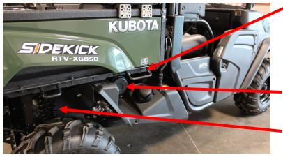
Tie-down hooks on both sides of the cargo bed for easy load security
