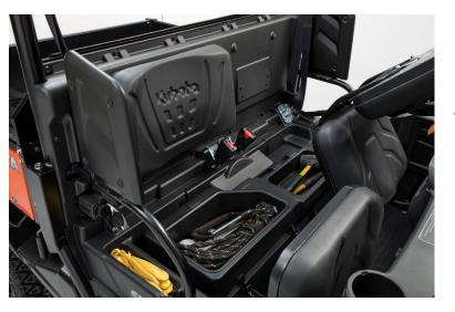
Large capacity storage compartments are provided under the split bench seat for ease of access and security
