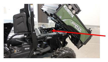
By starting a Walk-Around under the bed of the machine, we can begin by pointing out a main feature; the 48 hp gas engine with a flat torque band coming in between 4500 and 5700 rpm's. This engine was built for transport speed, cargo capacity, and towing.
