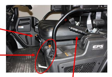
Hand operated rear wheel parking brake for safety and security when the machine is parked
